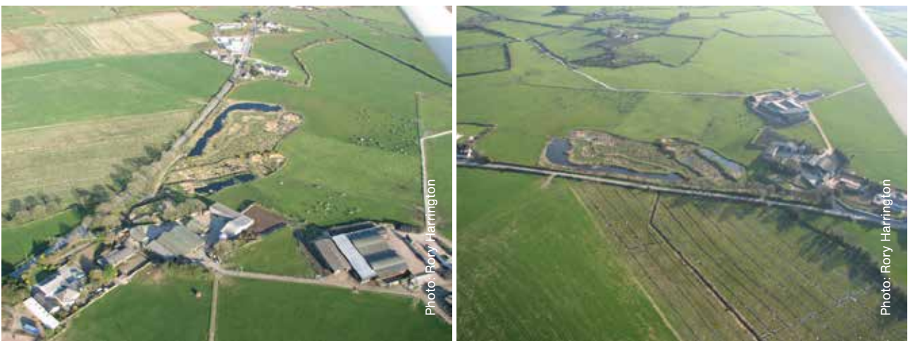
Figure 29. Integrated Constructed Wetlands (ICW) for treating farmyard waste waters in the Anne Valley catchment area, Co. Waterford.
